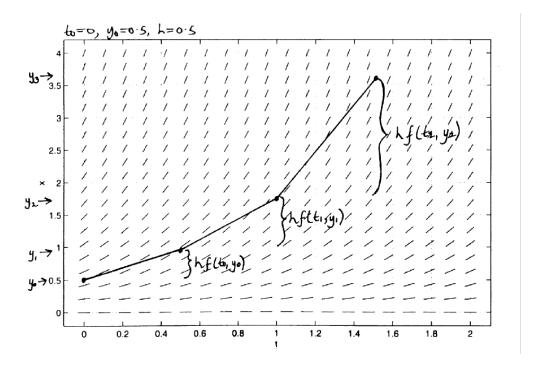
The next picture illustrates the relationship between the slope field and the numerical solution obtained with the Improved Euler method.
